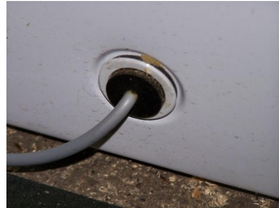
Insert Temp Probe via Drain Plug
