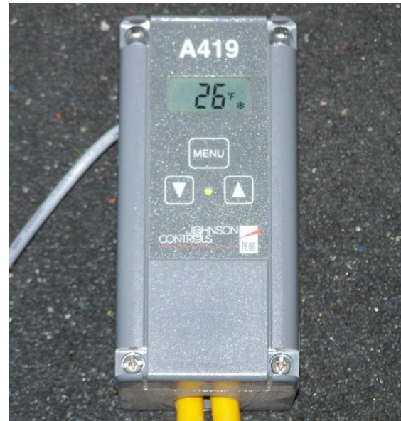
Johnson Controls External Thermostat
