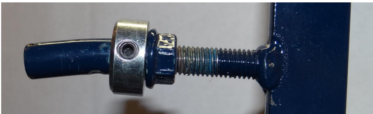
Figure 3. Ferrari floor corker insertion pin fitted with half-inch shaft-collar spacer in order to reduce the depth of Belgian beer corks in champagne bottles.
