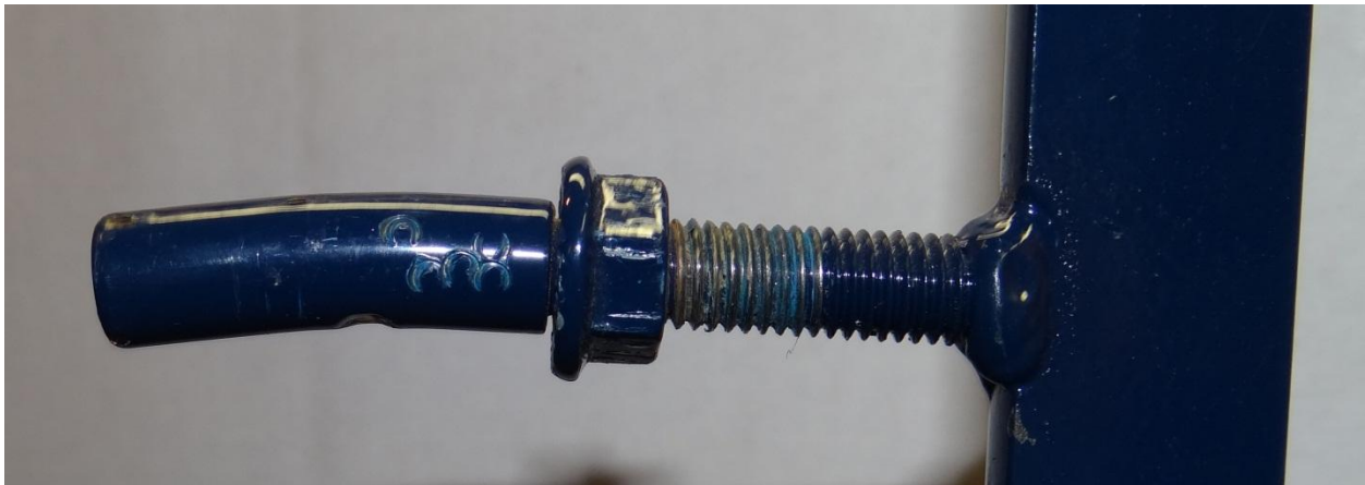
Figure 2. Ferrari floor corker insertion pin adjusted to minimal cork depth setting.
